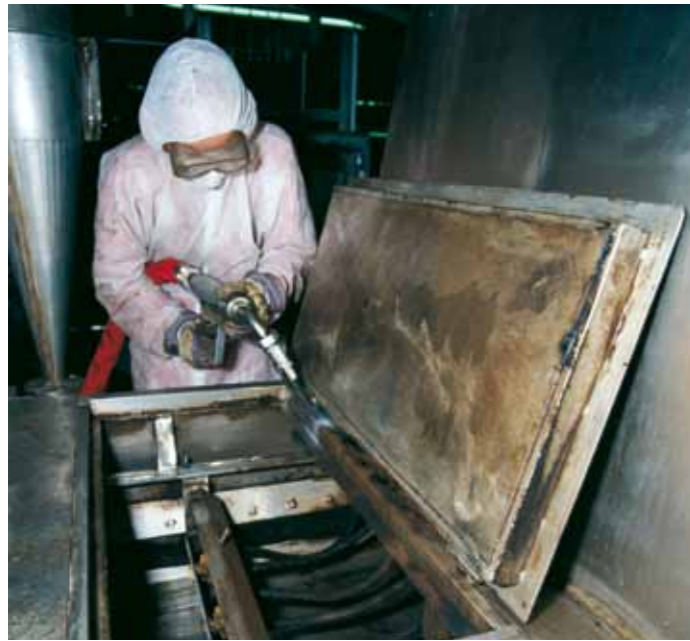
Cleaning a coffee production plant
