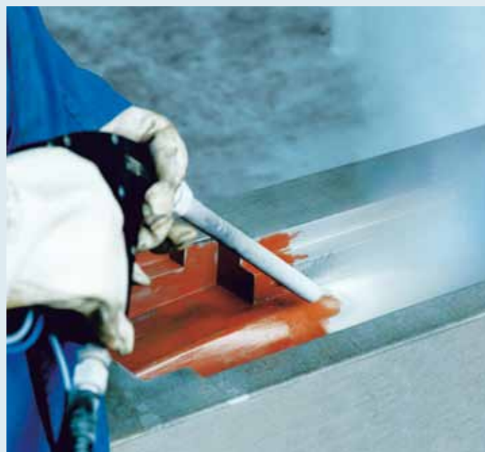
Dry ice blasting of a foundry core box
